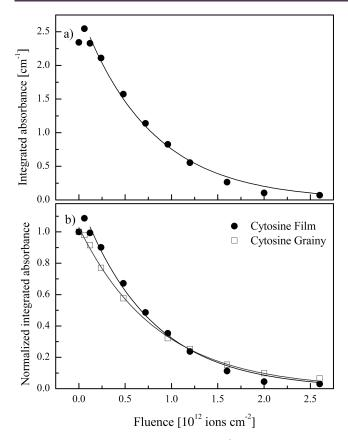
**Figure 3.** Integrated absorbance at 1539 cm $^{-1}$  of cytosine films as a function of the fluence of 17 MeV Ni $^{8+}$  (a). Normalized integrated absorbance at 1539 cm $^{-1}$  of the film (black circles) and grainy (open squares) cytosine samples as a function of the fluence of 17 MeV Ni $^{8+}$  (b).
