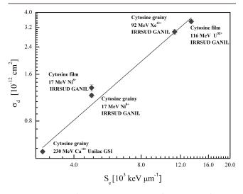
**Figure 6.** Apparent destruction cross section of cytosine as a function of the electronic stopping power.
