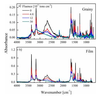
Figure 4. Spectra of grainy (a) and film (b) cytosine samples at 12 K. The samples were irradiated by 17 MeV  $Ni^{8+}$ at different fluences.
