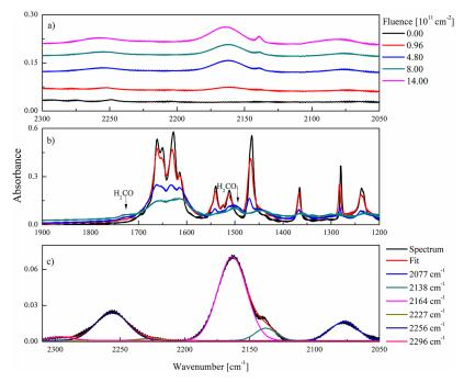
Figure 7. IR spectra of the cytosine film irradiated by 116 MeV  $U^{32+}$  at different fluences. The sample was irradiated by 116 MeV  $U^{32+}$  at different fluences, within wavenumbers ranging from 2300 to 2050 cm<sup>-1</sup> (a) and from 1900 to 1200 cm<sup>-1</sup> (b). Deconvolution of the band between 2300–2050 cm<sup>-1</sup> of the cytosine film irradiated by 116 MeV  $U^{32+}$  at the fluence of 1.44  $\times$  10<sup>12</sup> ions cm<sup>-2</sup> (19.6 eV per molecule) at 12 K (c).
