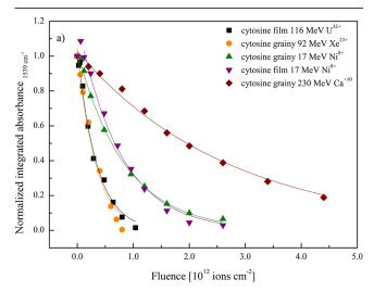
**Figure 5.** Normalized integrated absorbance at  $1539 \text{ cm}^{-1}$  as a function of the projectile fluence. The full lines correspond to the fitting of the data with eq 2.
